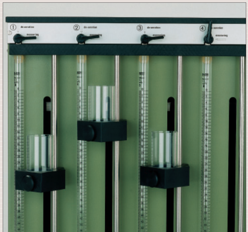
Buffer vessels of the calcimeter
